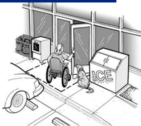
An accessible route to a door with maneuvering clearance maintained on the door's latch side makes entry possible for the customer who uses a mobility device.
